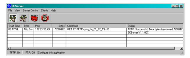
**NOTE:** The TFTP server process takes approximately 5 minutes, followed by an additional 30 minutes for the panel to be updated. During this time, it is common for the panel to experience various LED flashes and audible beeps from the panel.
