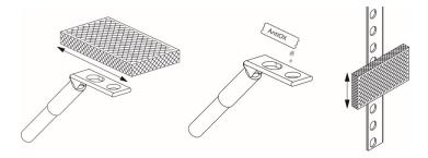
2. Next, attach the bent lug to the rail of the rack with thread-forming screws. (Once again, use of an AntiOx to cleanse the screws is recommended).
