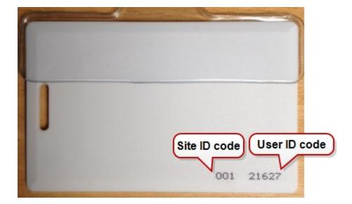
For 26 Bit cards the Gateway interface must be programmed for nine digits.
