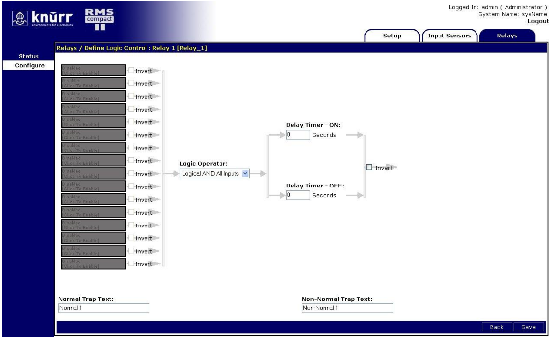
Figure 4-16. Relay Specific Configuration
