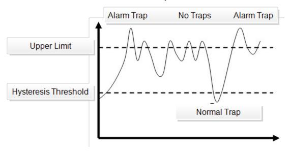
As shown in image above, the humidity first rises past its upper warning threshold, which generates an alarm trap.
