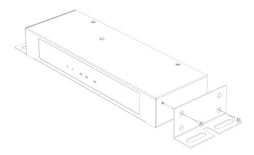
Hold the Gateway EP042 and attach the bracket to the rack using two 12-24 screws.
