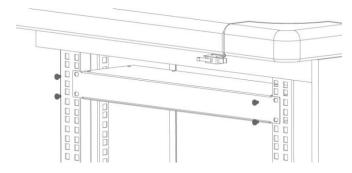
This product is intended to be installed using the racks RU mountings via the brackets found at either end of the rack PDU with mounting hardware provided.
