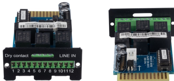
Figure 10: Relay Card Front and Top View (showing connection points)
