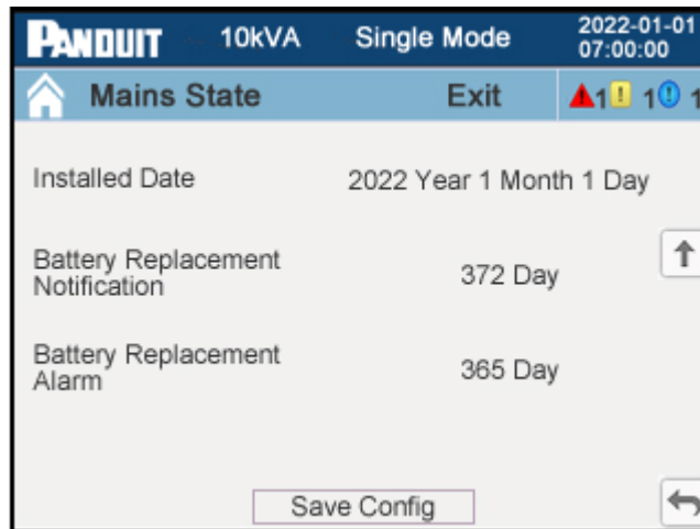
Figure 24I: Battery Setup Page 3 (3-Phase UPS)
