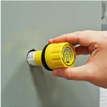
1. Insert the Indicator Module in the 30mm knockout hole, align anti-rotation notch. Ensure the rubber washer is on the outside of the enclosure.
