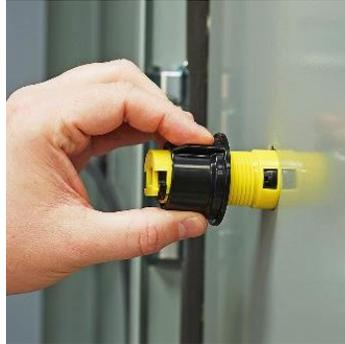
2. Install the panel nut with the flange towards the inside surface of the enclosure.
