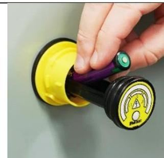
11. Install the battery. See Battery Replacement section of the manual for further details.
