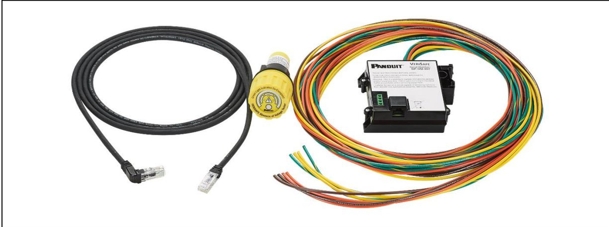
The VeriSafe Absence of Voltage Tester is a permanently-mounted tester that is used to verify a circuit is de-energized prior to opening an electrical enclosure. Once installed, a push of a button enables qualified electrical workers to verify the absence of voltage and see an active indication when the absence of voltage is confirmed. The Indicator Module is designed for a 30-mm notched panel knockout and the Isolation Module can be mounted to DIN rail or surface mounted using screws.
