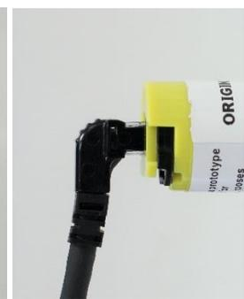
5. Insert the end of the AVT System Cable with the right-angle connector in the back of the Indicator Module. Press firmly into the opening until you feel it latch. Pull back on the connector to verify that it has properly latched.
