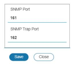
Figure 74: Setup SNMP Port and Trap Port
