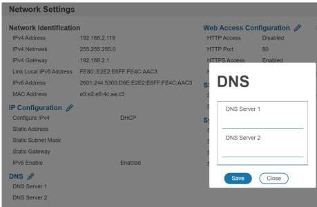
Figure 16: DNS Configuration
