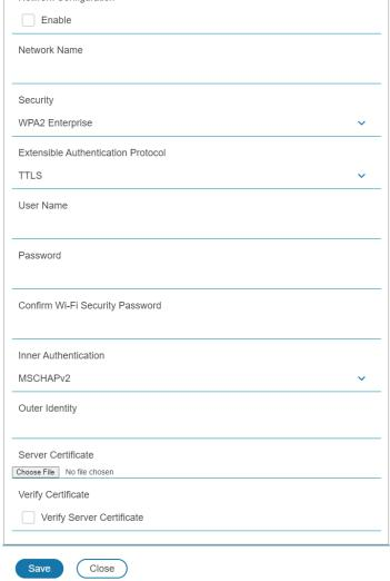
Figure 69: Wi-Fi Enterprise security Network configuration
