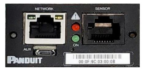
Figure 1: Ethernet Port for Network Connection
