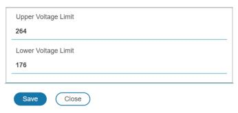
Figure 44: UPS Bypass Voltage Limit configuration
