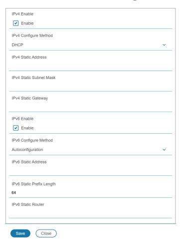
**Figure 15: Ethernet Interface Configuration**
