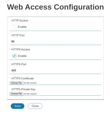
Figure 101: SSL Certificate Load Screen
