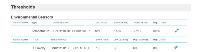
Figure 84: Environmental Sensor Threshold Configuration View
