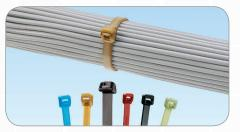
Secure cables with a selection of cable ties developed specifically for harsh environments, including polypropylene and nylon 12 (resistant to salts, acid rain and hydrocarbons) and Tefzel<sup>▼</sup> and PEEK (Polyetheretherketone) (withstand high temperatures).
