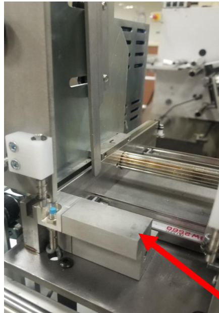
Figure 4 Long Plate Support Block Installed
