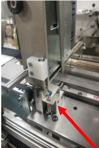
Figure 3 Cale support de plaque courte installée
