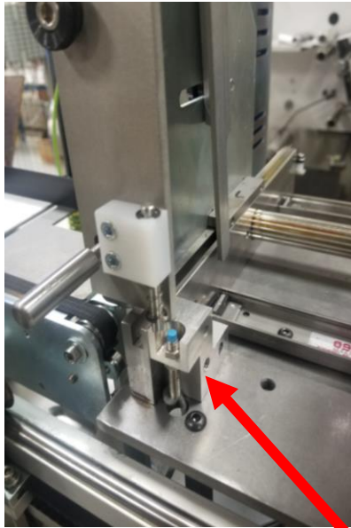
Figure 3 Bloc de support court installé
