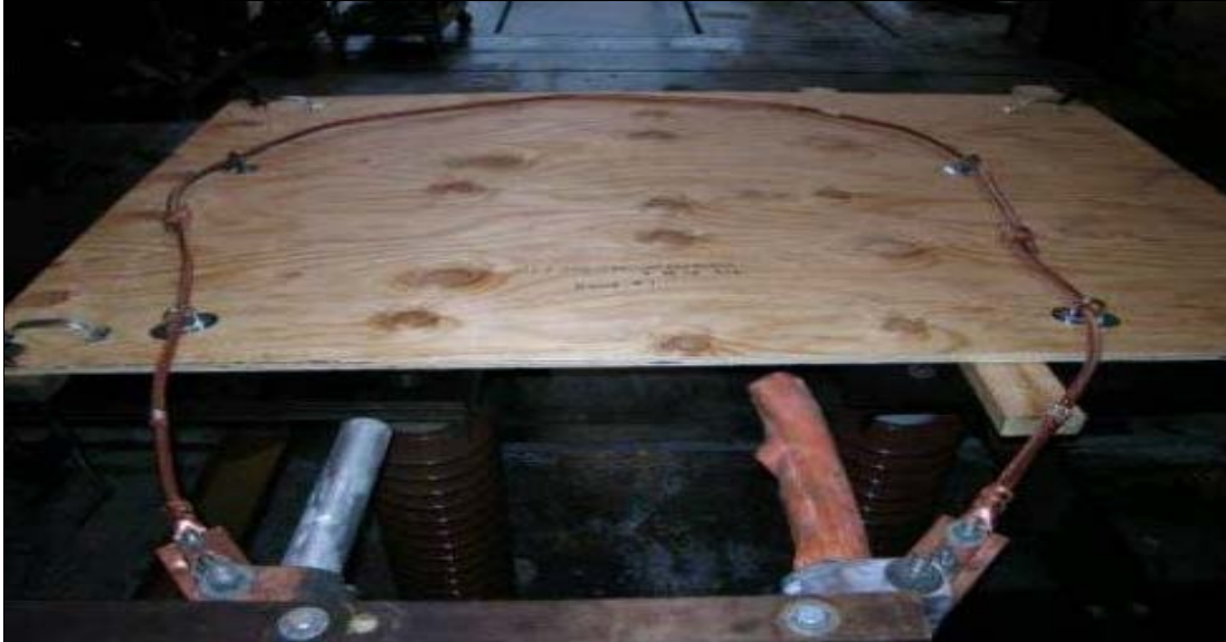
Figure 3. EMF test setup at Powertech Labs. Current values ranged from 3.7kA RMS to 70.9kA RMS .
