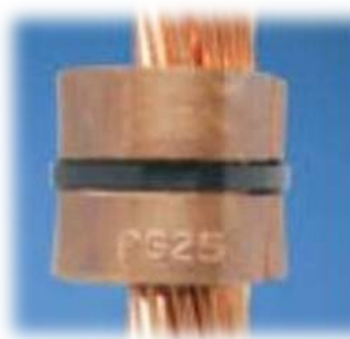
Part crimped one time embosses die numbers once
