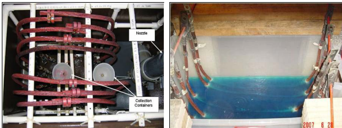
Figure 8. Corrosion test setup groups. Salt spray (left) and acid tests (right).
