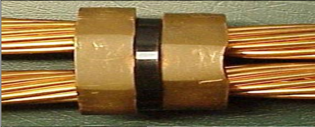
Figure 13. Connector crimped through steps one and two, showing the additional compression achieved by the enhanced crimping process.
