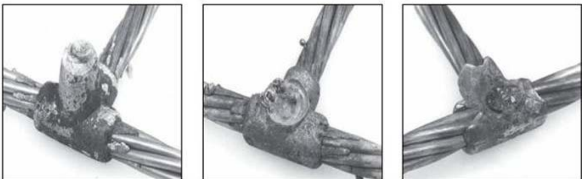
Figure 17 - Good and bad exothermic welds. It is difficult to tell the difference between acceptable and unacceptable connections.
