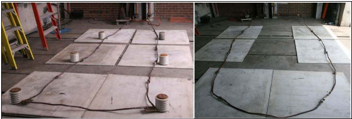
Figure 9. Fault current test layout for the acid sequence and salt spray samples.
