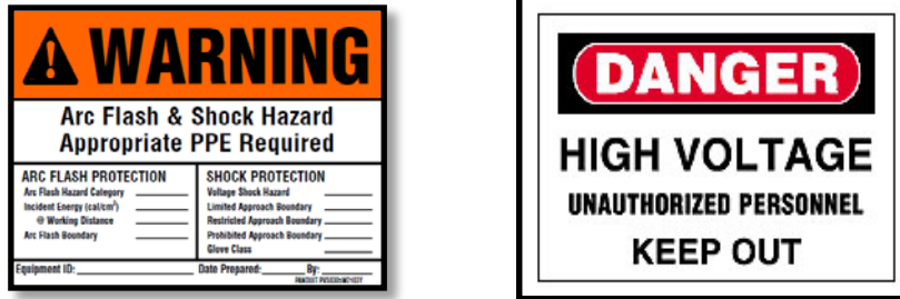
Figure 6. Example of an arc flash warning label and high voltage safety sign that meet the 2012 NFPA 70E requirements.
